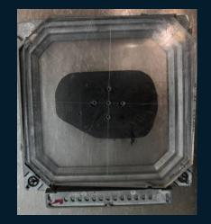
• The black block is the 3D printed mould that would be used to mount onto the acrylic plate.
